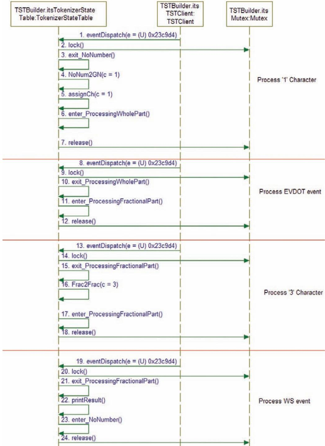
Figure 5-17: State Table Pattern sequence for execution of “1.3” string
